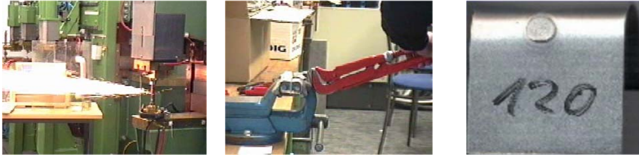
Figure 1: a) metal objects are joined using resistance spot welding, b) the welding joint is torn apart in a destructive test, c) quality is estimated from the diameter of the welding joint.
