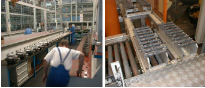
Figure 8. Assembly of hydraulic pumps
